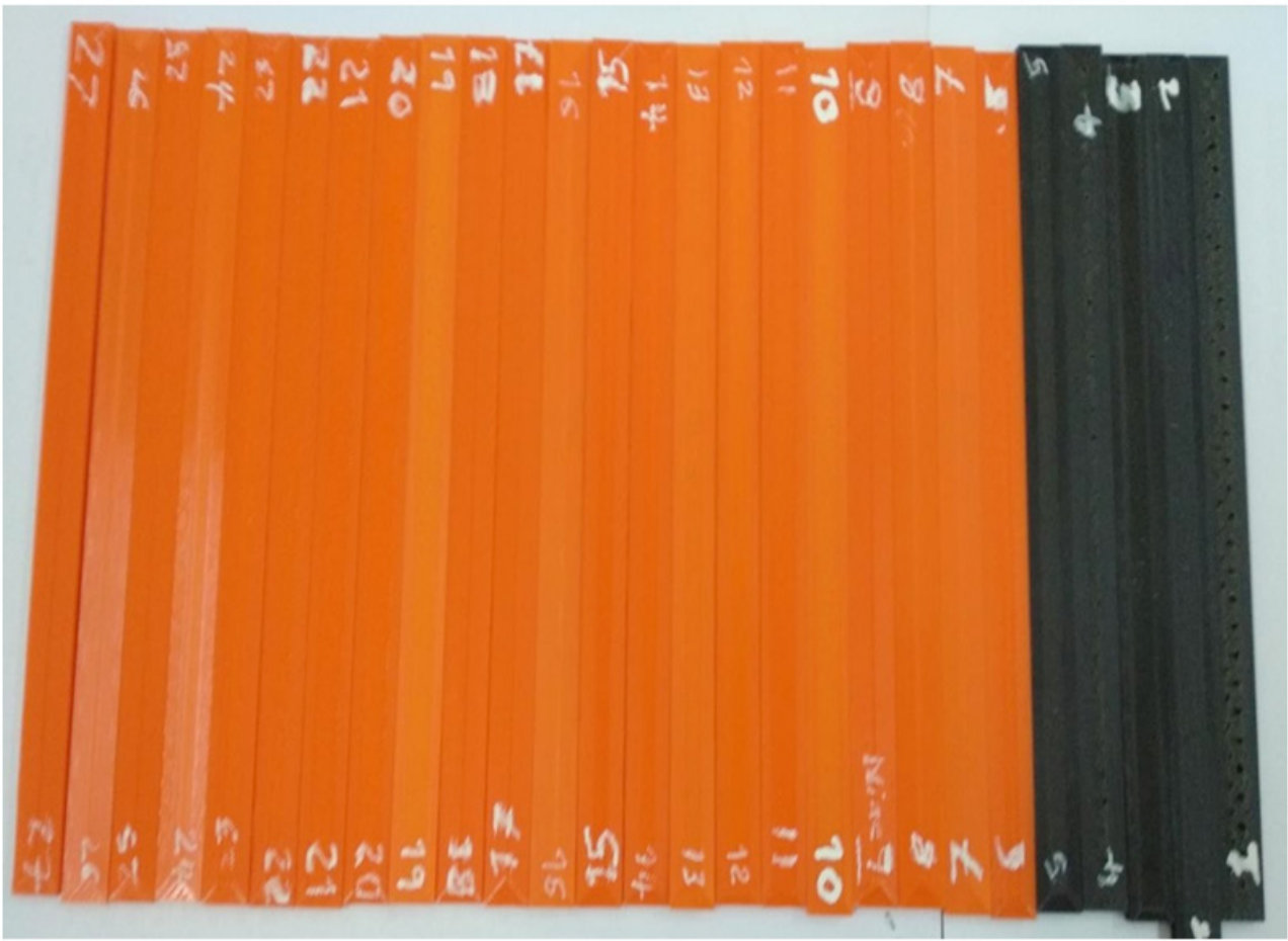
Figure 2: Rectangular workpieces after fabrication on FDM machine
