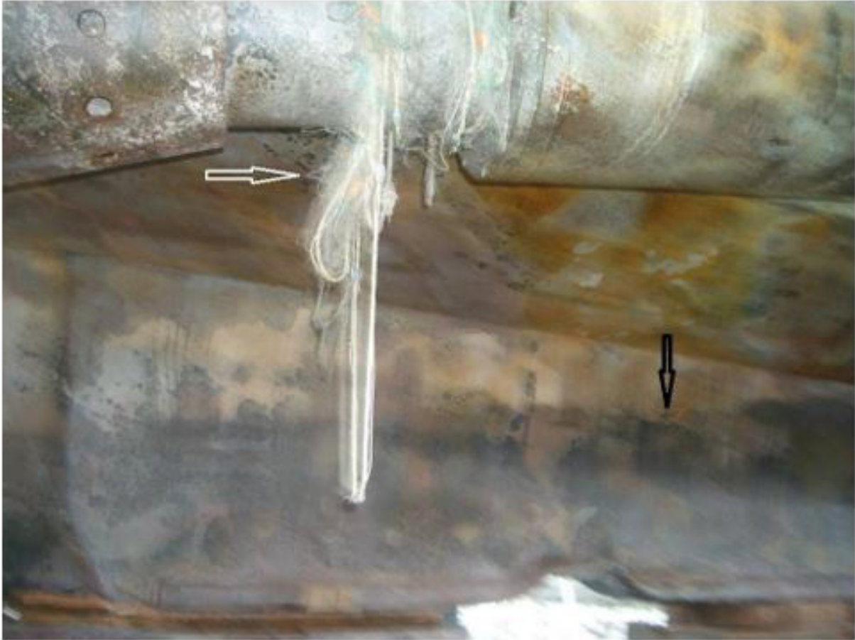
Figure 11: The tangled fishing net wires (white arrows) on the propeller axis indicate the running aground prior to the explosion and the black charred hull surface (soot) may be due to the flame at the moment of the blast for an underwater explosion (black arrows). Also, it cannot be ruled out that the strong ICCP current might flow on the hull surface when it ran aground before the underwater explosion [3,7]
