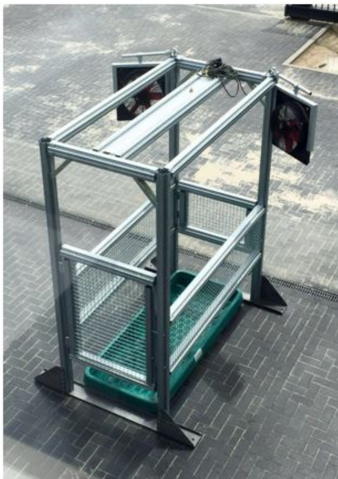
Figure 1: An example of the ECU, equipped with a special sprinkler on top, and two fans at the back poles.
