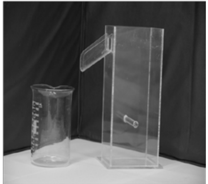
Figure 1: The hand and wrist are submerged in the hand volumeter (right) and the mass of the fluid is displaced to a weighed beaker (left) is multiplied by the density of the water-3% ethanol mixture. The middle and ring finger are separated by a plastic peg in the volumeter.
