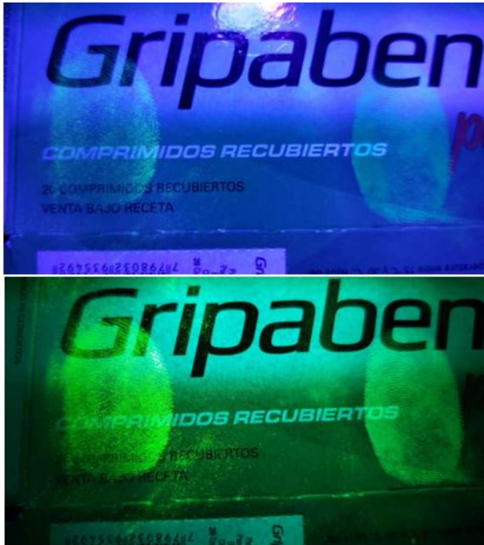
Figure 17 and 18: Fingerprints developed with phosphorescent powder (left) and with fluorescent powder (right), without using ultraviolet filters (above) and with ultraviolet filters (below)
