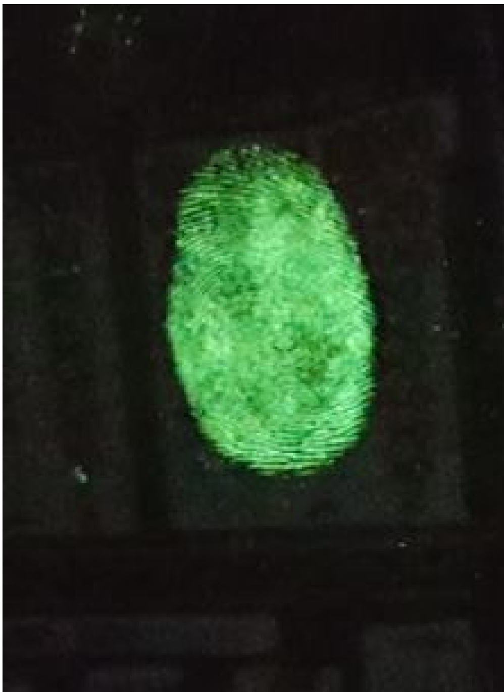
Figure 9: Fingerprint developed with phosphorescent powder (left) and with fluorescent powder (invisible, on the right) once the light source has been turned off
