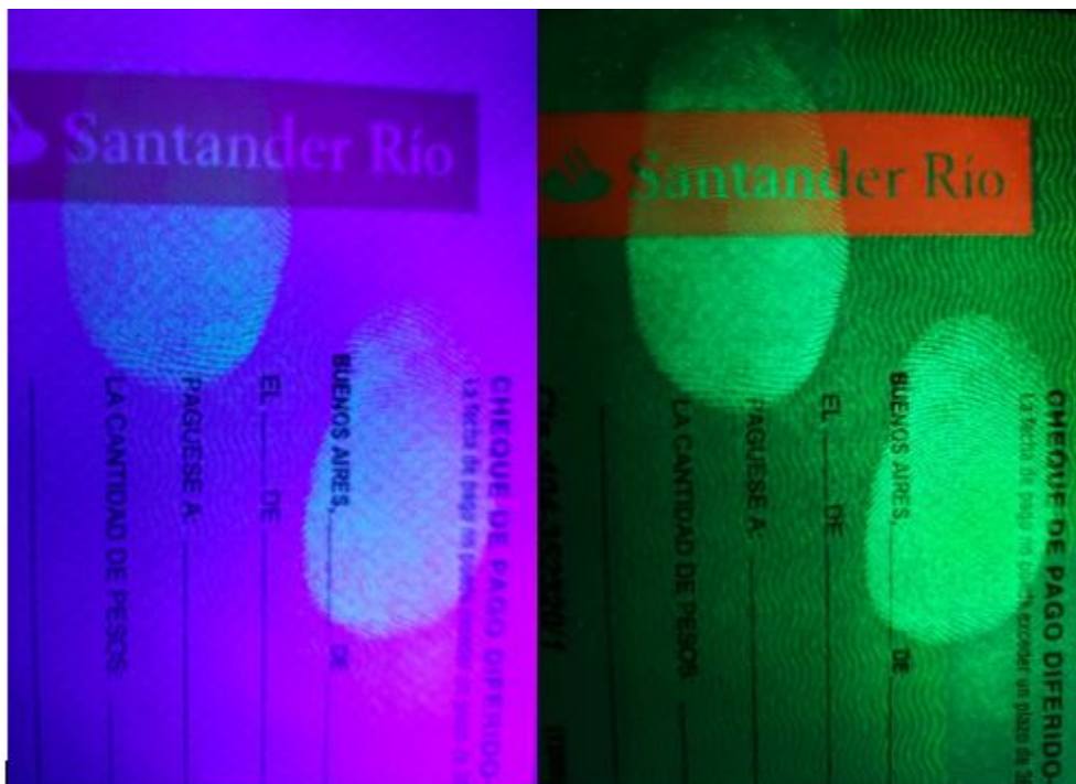
Figure 14: Detail of fingerprints developed with fluorescent powder using ultraviolet light without filter (left) and with ultraviolet filter (right). No contrast was visualized when the light source was turned off
