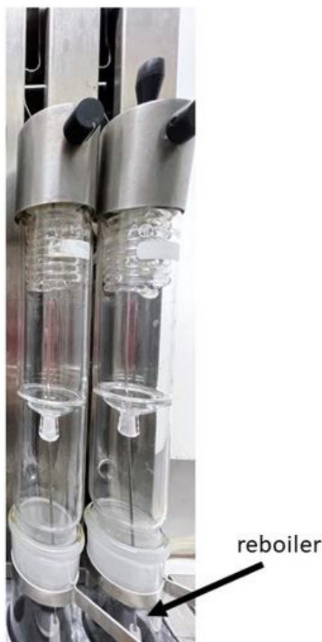
Figure 1: Photograph of Reboiler
